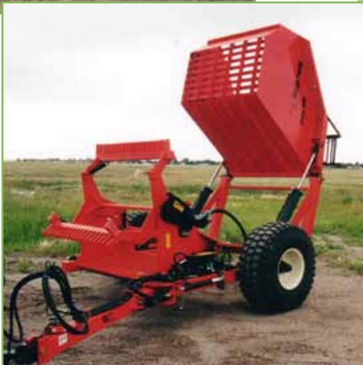
The RR900ST hopper lifts up to 60" for dumping.
