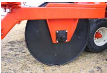
< Heavy duty bearings complete with replaceable shaft
