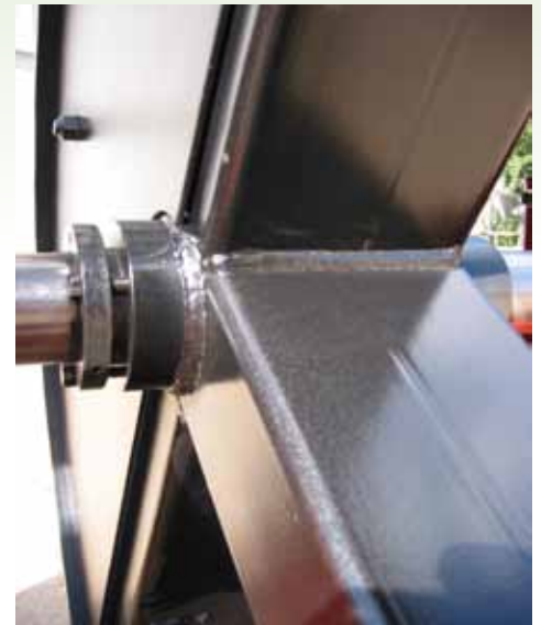
> A bolted end cover plate allows access to the inside of the replaceable shaft. A tapered keyed hub centres the replaceable 2 7/16" shaft on 6" x 3" structural tube cross members.
