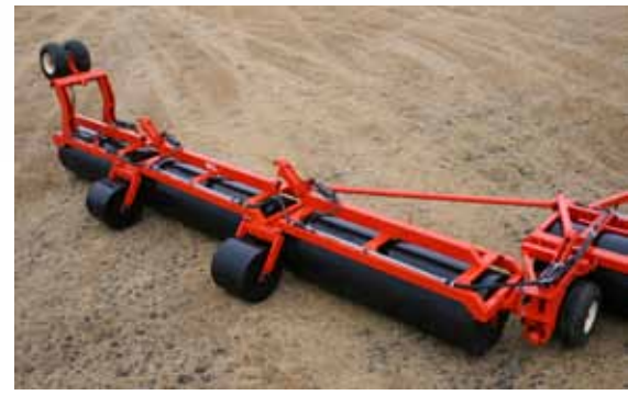
Each roller uses a large, 4-way heavy duty and flexible universal joint to allow each roller to float independently while maintaining constant ground pressure over changing terrain.
