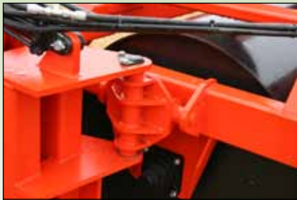
< Each extra large universal joint uses induction-hardened chrome-plated pins.
