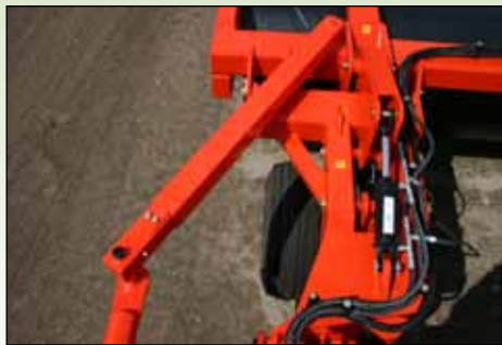
^ Telescopic draft arm allows narrow transport, even while turning sharply.
