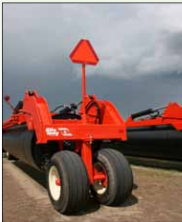
^ Pivot wheel in transport mode. The slow-moving vehicle sign also serves as a wheel-angle indicator when unfolding.
