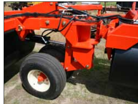
^ The finishing rollers are the key to the flexibility of Rite Way's land rollers, and to the narrow transport width.
