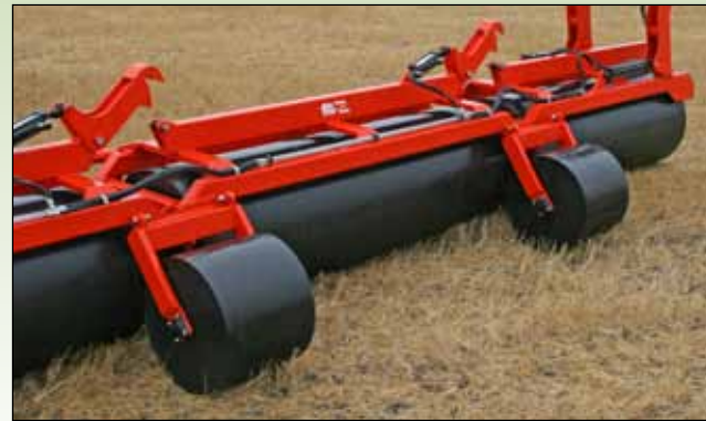
^ The finishing rollers are the key to the flexibility of Rite Way's land rollers, and to the narrow transport width.
